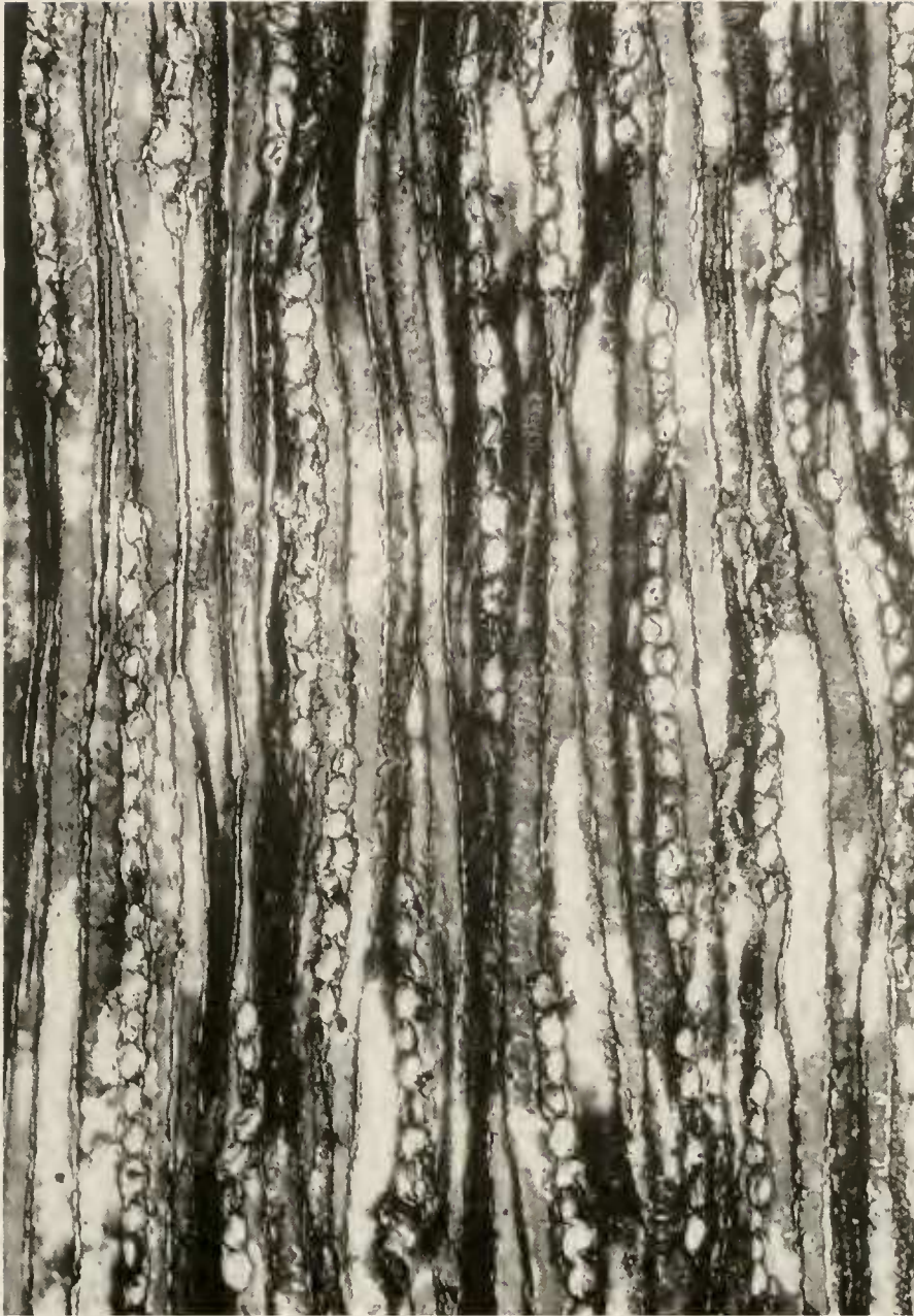
Fig. 8. Tangential longitudinal section with homocellular predominantly uniseriate rays. x 115.
